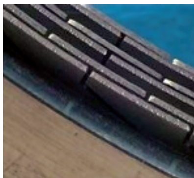
Figure 6: detail of finger seals showing offset.
